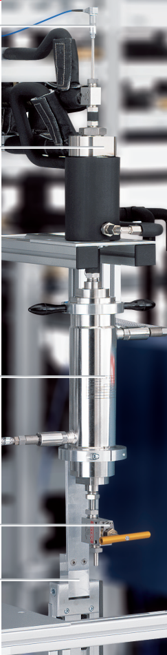
Option «Fractionated Separation» with high-performance fluid cyclone. Collecting basket is equipped with a lifting device for easy handling.
