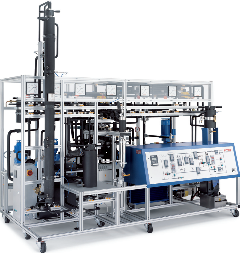
Multi-purpose SFE pilot unit for solid and liquid raw materials built for 500 bar max. operating conditions designed for research (Russia). The system includes the options fractionated separation with fluid cyclone, modifier system and Coriolis mass flowmeter.
